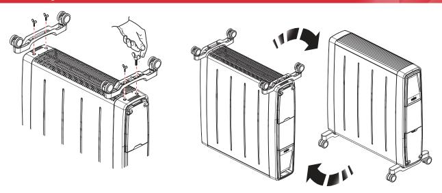
**WARNING -** The radiator must only be operated with the wheels and castors securely fitted and in the upright position.
