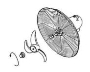
6. Slot the fan blades (4) on to the motor shaft (7) by aligning the D shaped hole on the blades with the shaft. Secure by attaching the blade cap nut (3) and turning anti-clockwise.
