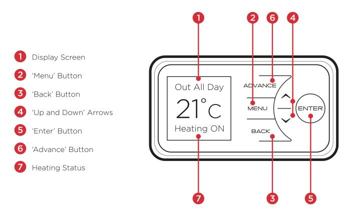
The heater is fitted with an adjustable thermostat enabling the room temperature to be controlled. The minimum room temperature is 7°C. The maximum temperature is set to 26°C by default. The minimum and maximum selectable temperatures available on the heater can be adjusted in the settings menu. A temperature of 21°C is a common comfortable room temperature.
