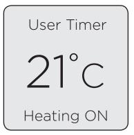
When the heater is in a timer profile and trying to achieve or maintain a room temperature, 'Heating On' will be displayed, otherwise, 'Heating Off' will be displayed. The words 'Heating On / Off' will not be displayed in a manual mode of operation.
