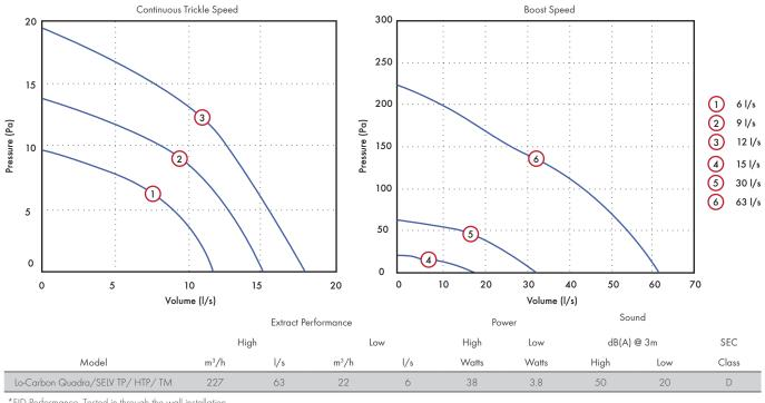
\*FID Performance. Tested in through the wall installation
