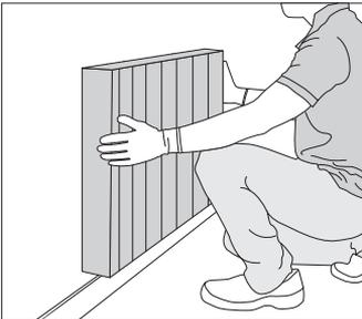
5. Slide product into fixed brackets, using a top to bottom method. Lift the product higher than the bracket and slide downwards into position.
