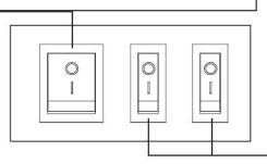
HEATER SWITCH: If only one of the heater switches are on, the units heating power is 1.5kW When both heating switches are turned on, the heating power is 3kW. When the heater switch or heater switches is/are turned on, the heater switch light(s) will illuminate. When the heater switch or heater switches is/are turned off, the light(s) will go off.
