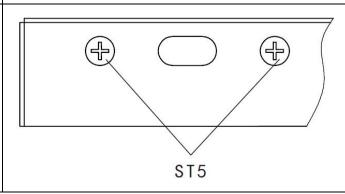
6.2 Mount the air curtain onto the installation bracket, choose suitable fixing holes in according to the need of air flow angle and then tighten with M5\*16 bolts.
