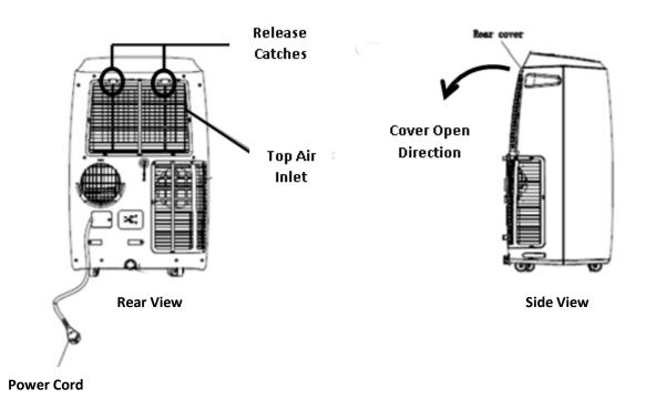
2. Insert the filter into the aperture in the rear of the unit that has been revealed by removing the top air inlet cover. Note the filter should be orientated so the small plastic bracket is positioned in the top left-hand corner and facing towards the top air inlet cover (see below). When inserting the filter avoid touching any of the exposed cooling coils/fins in the rear of the unit. Make sure the filter is securely fitted in the aperture before refitting the inlet cover.
