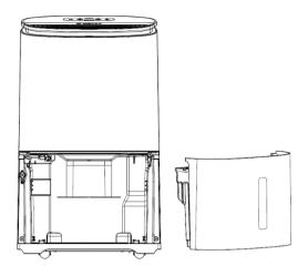
Step 1: Remove the water tank.
