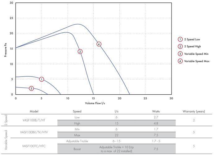
All performance testing was done in "through the wall conditions" - installed with 400mm rigid ducting and an exit terminal.
